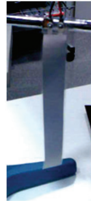
PVDF film hanging on the support to harvest the energy from the wind and temperature fluctuations of the environment. PVDF is a pyro and piezoelectric polymer.
