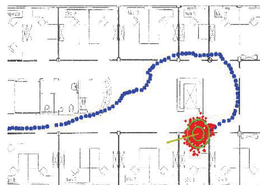
Fig 4: Tracking of a walking person in the HSG-IMIT lab
