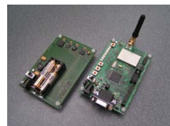
Fig 2: Nanotron Development board with HSG-IMIT sensor board extension
